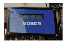
The weighing indicator will show the weight of each weighing tube. The accuracy of the weight is 5 grams.
